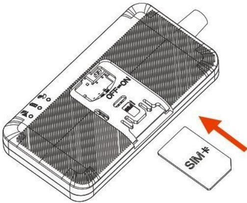
Note: SIM card should be equipped with GPRS and SMS functions.
